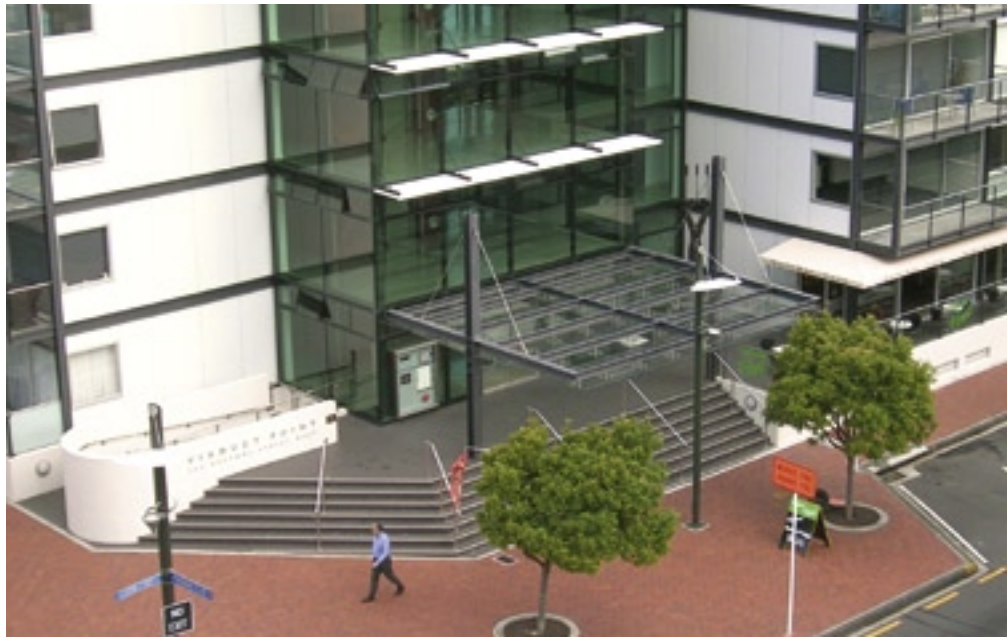
The corner location, generous steps and large canopy all help clearly signal the entry to this apartment development.
