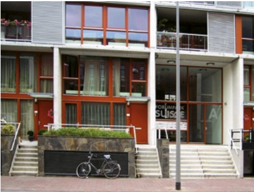
Ground floor apartments are here raised above street level and ventilation grilles for underground parking are well-incorporated into street edge design.
