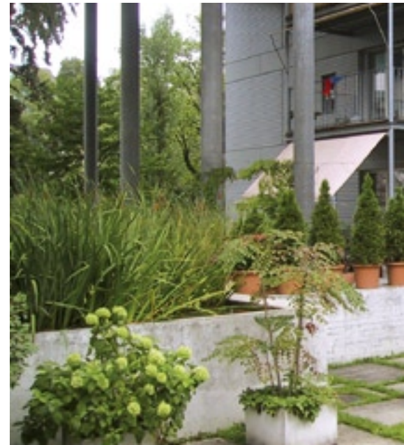
In this situation a change in level and a water pond planted with rushes (to the left of photo) is used to define the boundary between the private open space of ground floor units and a public driveway that runs past. Occupants here have used planters and pot plants to increase privacy & further define their territory. Balconies have similarly been adapted with screens for greater privacy.
