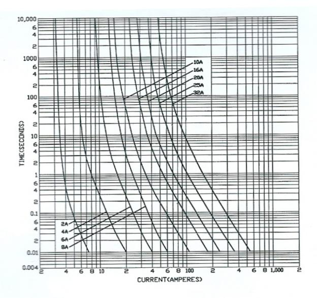
(i) Refer to inverse time graph and determine how long it will take for the 32A HRC fuse to operate with the fault current calculated in (a)(iii) flowing.
