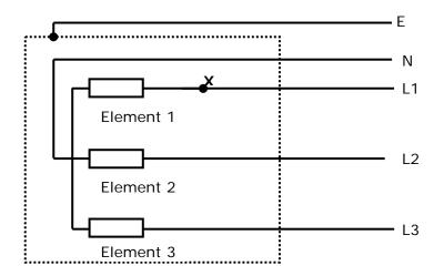
An earth fault of negligible impedance has developed between L1 and the oven frame while the oven is operating. The fault occurred at point X.
