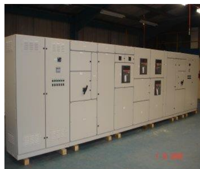
Multi-cubicle type assembly
